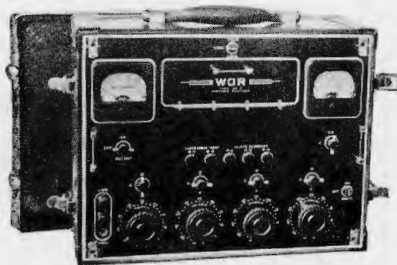
UTC HIPERM ALLOY AUDIO TRANSFORMERS are used in the new WOR 30B portable amplifiers (Front and back view illustrated) for use in remote pickup broadcasts in conjunction with the new WOR high fidelity 50,000 watt transmitter.
